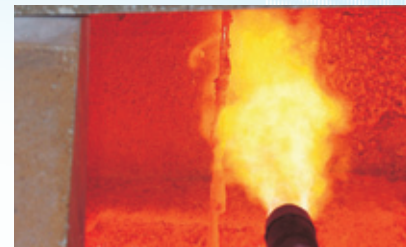
Sapphire temperature probe in a glass furnace
