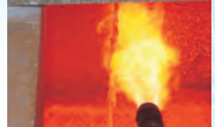
Sapphire temperature probe in a glass furnace
