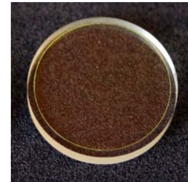
5 μm thin YAG:Ce screen
